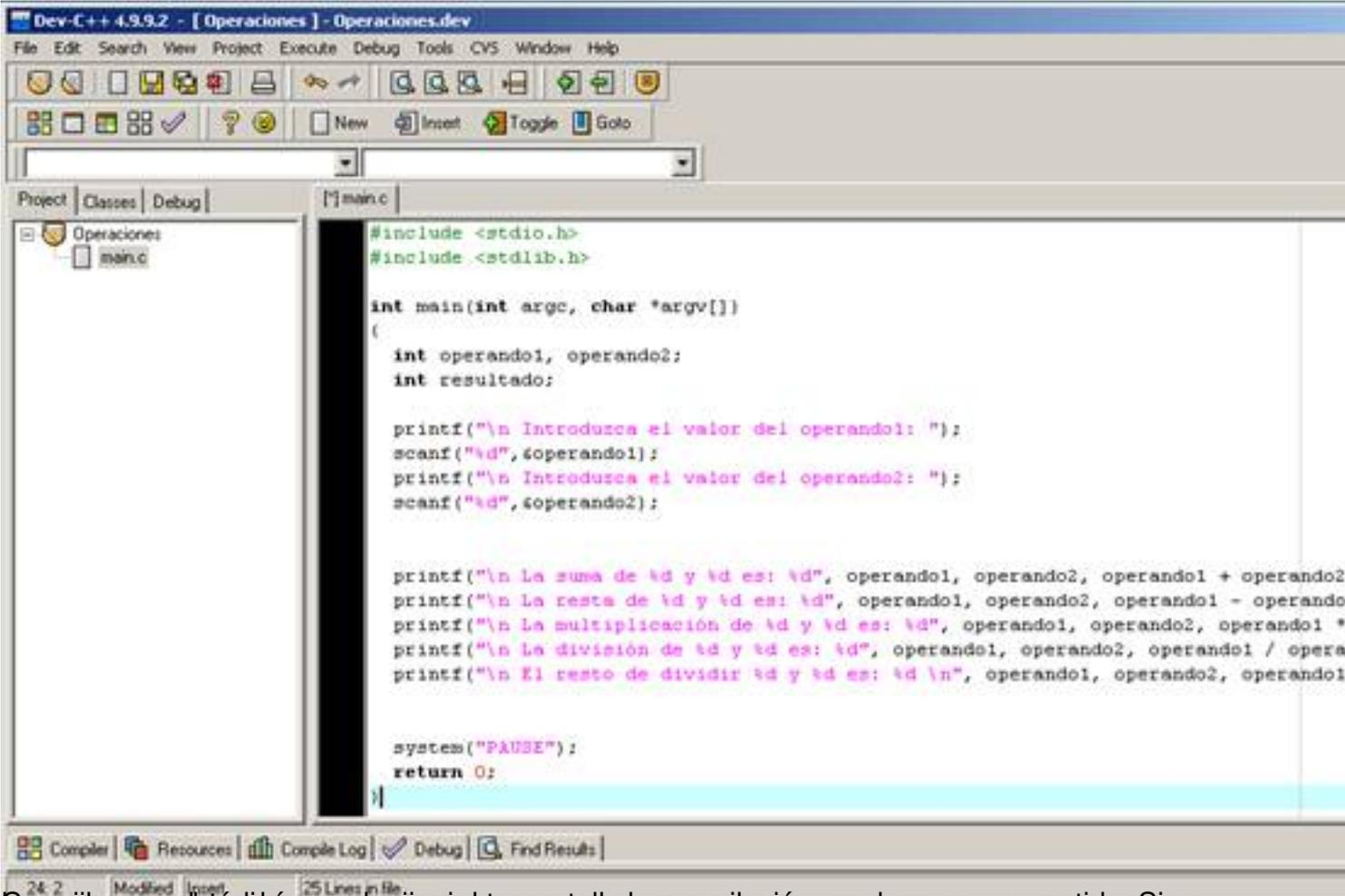
The screenshot shows the Dev-C++ 4.9.9.2 IDE with a project named 'Operaciones'. The main window displays the source code for 'main.c'. The code includes headers for `<stdio.h>` and `<stdlib.h>`. The `main` function takes two integers as input, performs addition, subtraction, multiplication, and division, and prints the results. It also includes a `system("PAUSE");` call to keep the window open.
